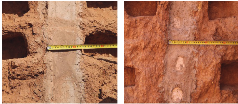
FIGURE 5: Macroscopic shapes of the fissure after grouting: (a) traditional and (b) optimized.
