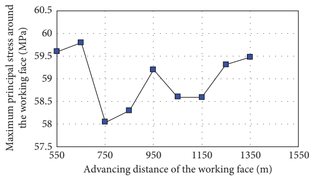
FIGURE 7: Relationship between the maximum principal stress around the working face and the advancing distance.
