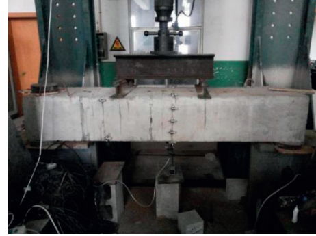
FIGURE 3: Loading equipment and methods of static load.
