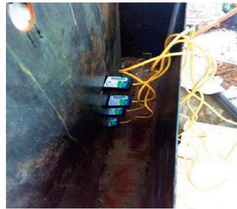
FIGURE 8: Moisture tester layout.
