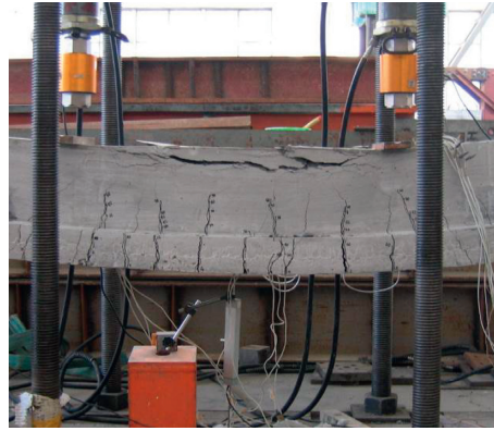
FIGURE 12: Cracked test beam SCB-1.
