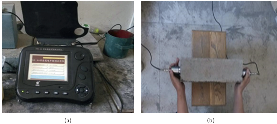
FIGURE 1: NM-4A nonmetal ultrasonic detection analyzer.
