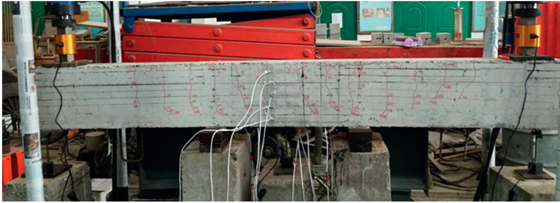
FIGURE 2: Actual RC beams with 600 MPa steel bars and the test device.
