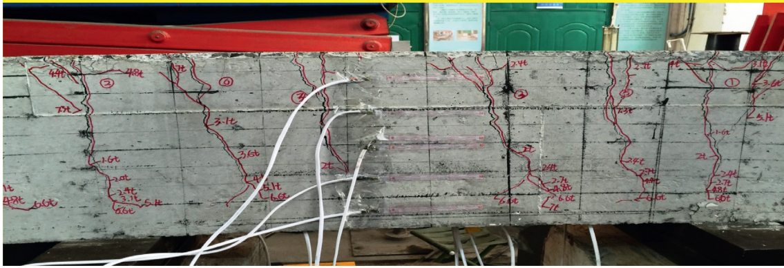
FIGURE 4: Actual failure mode of the RC beam.
