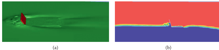
FIGURE 5: Simulation results of 60° floating plate. (a) 60° free waveform diagram. (b) 60° volume fraction diagram.
