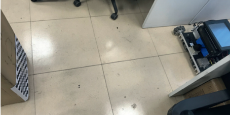
FIGURE 2: Calibration is performed using a calibration plate affixed to a prominent raised surface.
