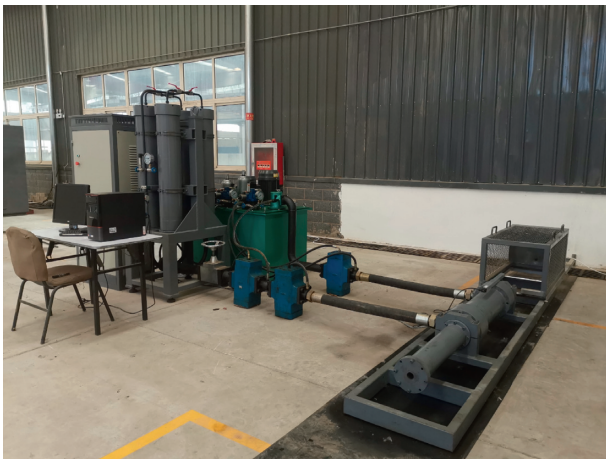
FIGURE 9: 300 kN test bench.
