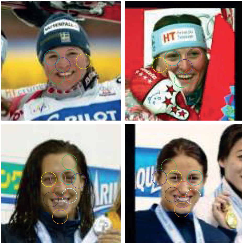
FIGURE 18: Face image FE and matching. Different colored circles in the same picture indicate different extracted features, and the same color in different pictures in the same group indicates matching similar features.
