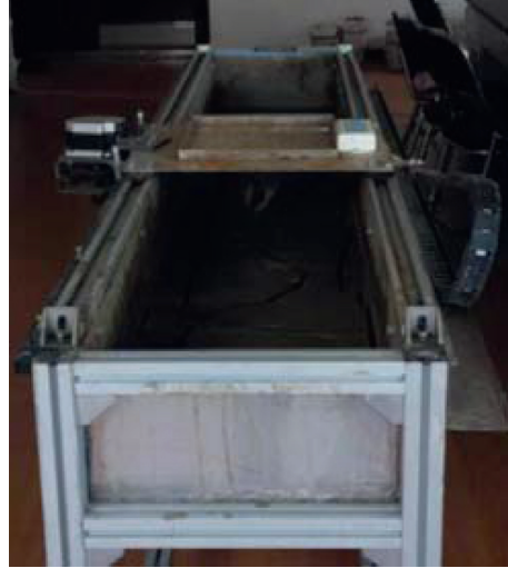
FIGURE 16: The test soil bin.
