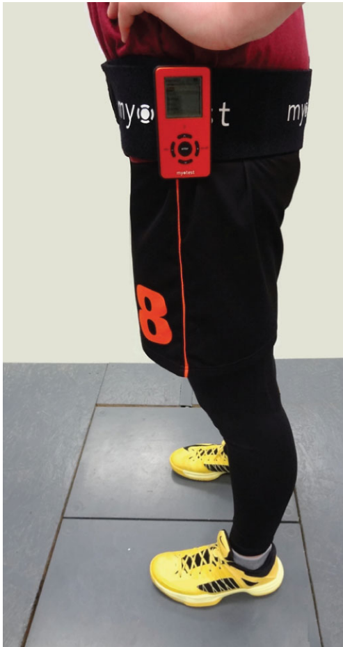
FIGURE 1: One of the participants standing on the force plates with the belt to which the Myotest accelerometer is attached vertically on the left side of the body at the pelvic level.
