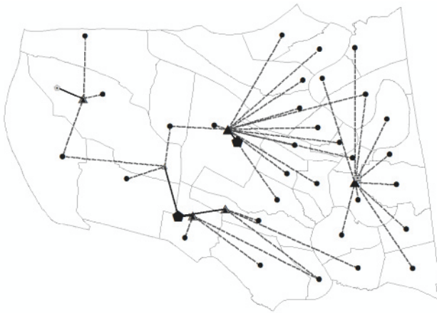
Optimal layout of MSWM system under cost objective
