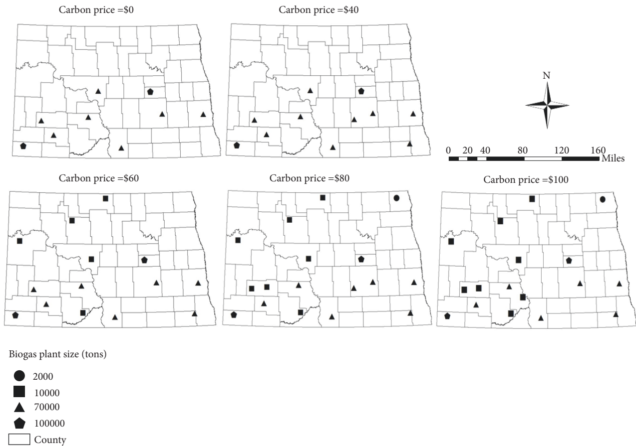
FIGURE 6: Impact of carbon price on biogas plant locations and sizes.
