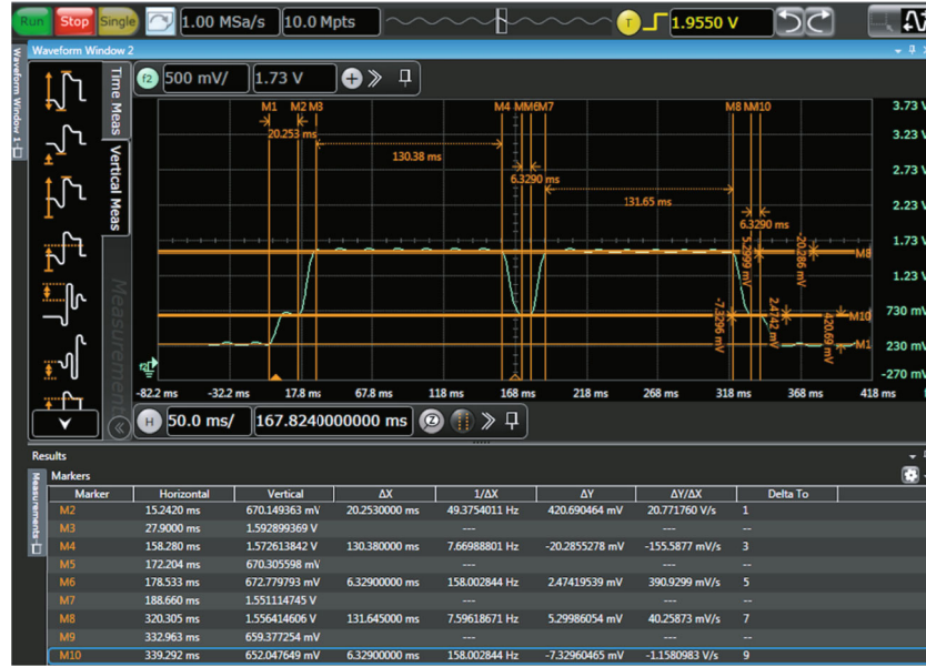
FIGURE 14: Current consumption of eMeD during active and idle modes.
