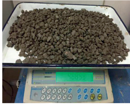
FIGURE 1: RAP material after drying and sieving.
