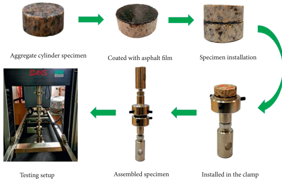
FIGURE 6: Flow chart of pull-off test.
