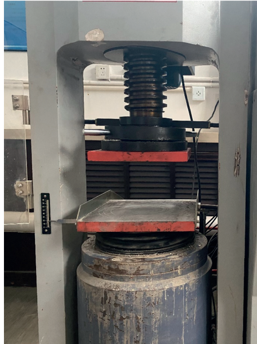
FIGURE 2: 2000 kN press machine.
