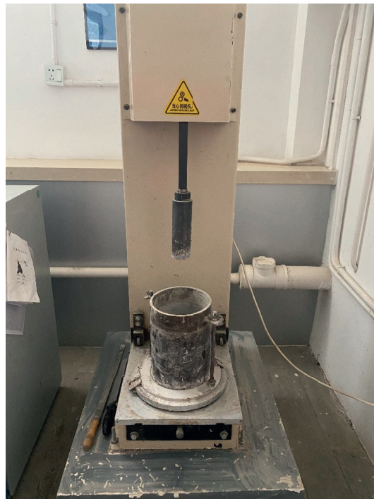
FIGURE 1: Compaction test apparatus.
