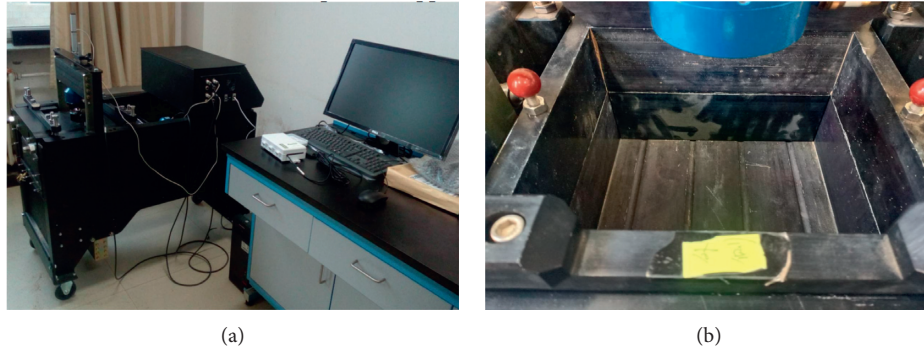
FIGURE 3: Large direct shearing instrument. (a) Large direct scissor photos. (b) Upper and lower shear boxes.
