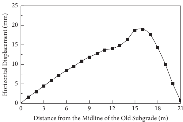
FIGURE 8: Horizontal displacement of subgrade top surface.
