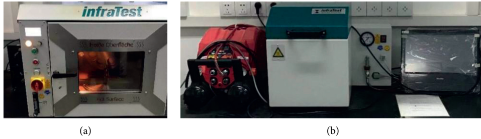
FIGURE 1: Aging instrument for asphalt binder. (a) RTFOT. (b) PAV.
