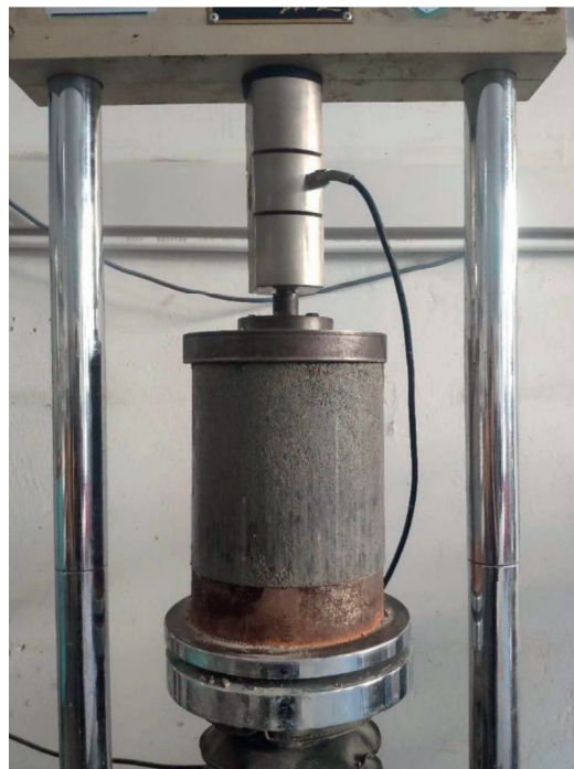
FIGURE 3: Pavement material strength tester.
