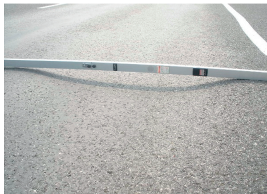
FIGURE 7: Result of the rutting survey at sample 5.
