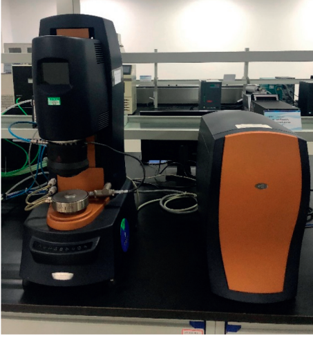
FIGURE 2: Kinexus ultra + rotational rheometer.
