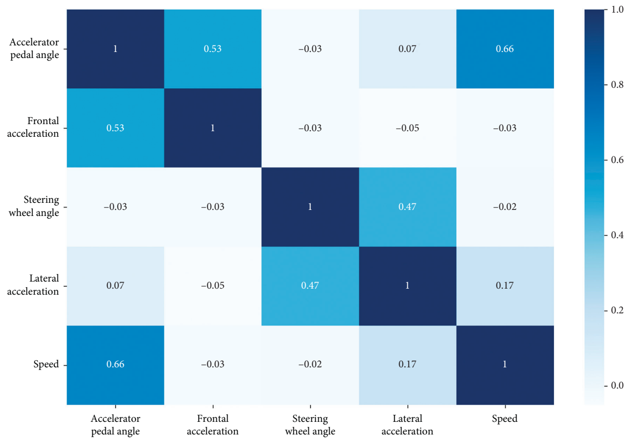
FIGURE 5: A matrix showing the correlation between the five signals acquired from the CAN bus.
