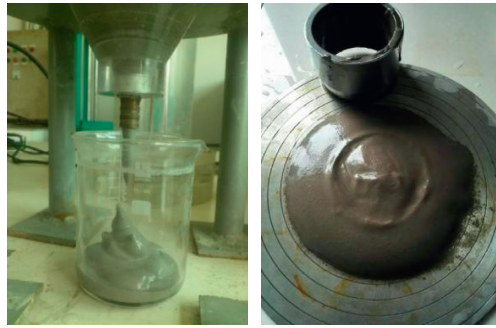
FIGURE 6: Underflow of dynamic thickening test.
