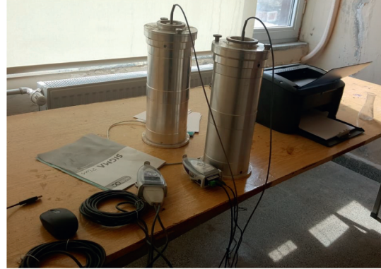
FIGURE 5: The measurement of computer-controlled hydration temperature in the blended cement.
