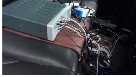
FIGURE 22: Digital acquisition hardware inside the car.
