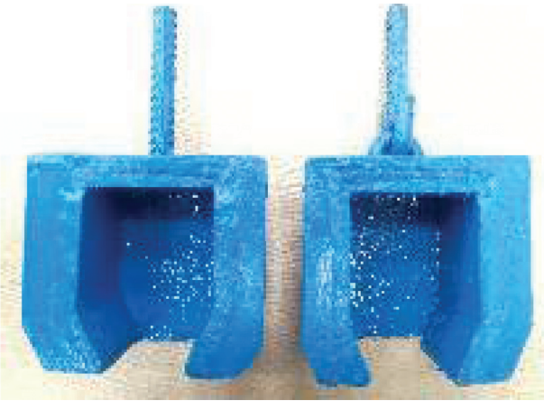
FIGURE 4: Special fixtures used in the uniaxial tensile test.
