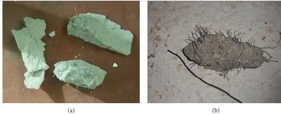
FIGURE 7: Fractions of SFRC members: (a) MTF25-0.77; (b) MTF25-N.
