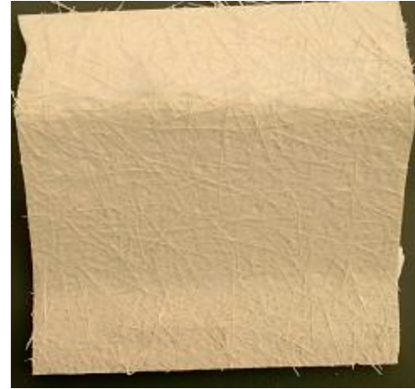
FIGURE 1: Sample of GFRPA waste.
