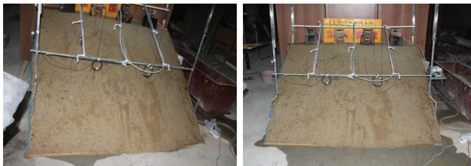
FIGURE 11: Fiber optic strain experiment under different rainfall conditions.
