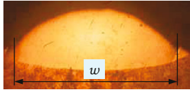
FIGURE 2: Geometry of section of single-track formation.
