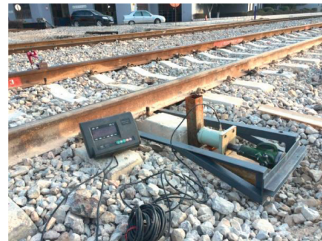
FIGURE 6: Lateral resistance test of sleeper.
