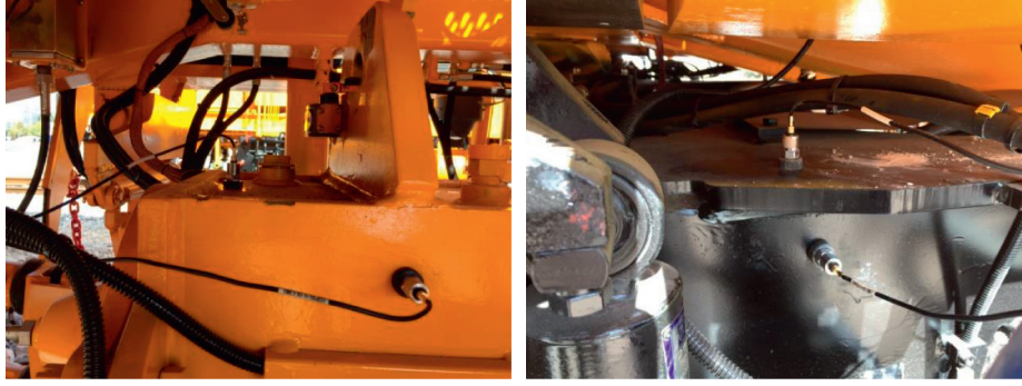
FIGURE 3: Sensor installation on the stabilizing device and bogie.
