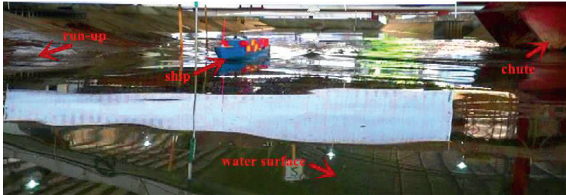
FIGURE 7: Interaction process between ship and landslide-induced wave.
