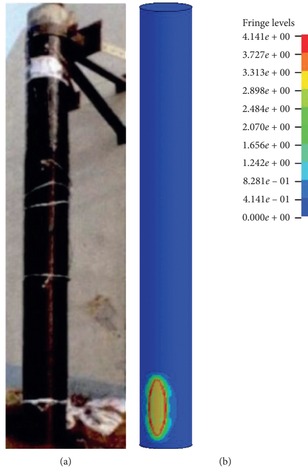
FIGURE 8: Deformation of tested column. (a) Test result. (b) Numerical result.
