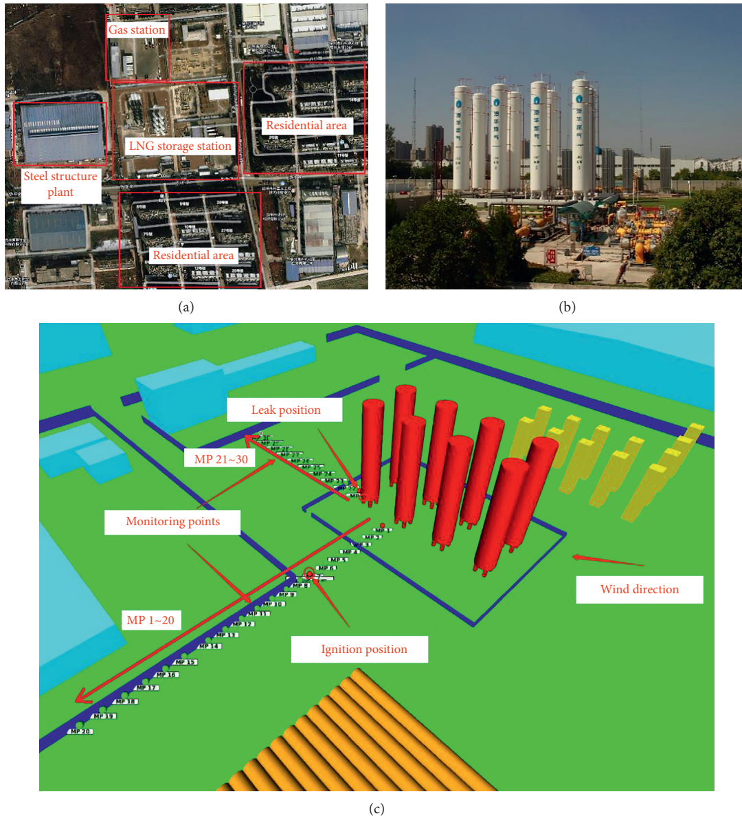
FIGURE 2: Developed numerical model of the LNG accidents: (a) satellite topographic map; (b) LNG storage tank; (c) information of numerical model.
