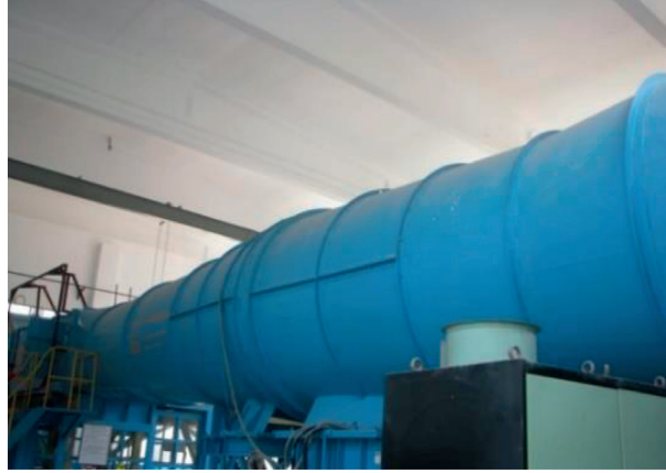
FIGURE 3: Wind tunnel with low wind speed (1.4 m × 1.4 m).
