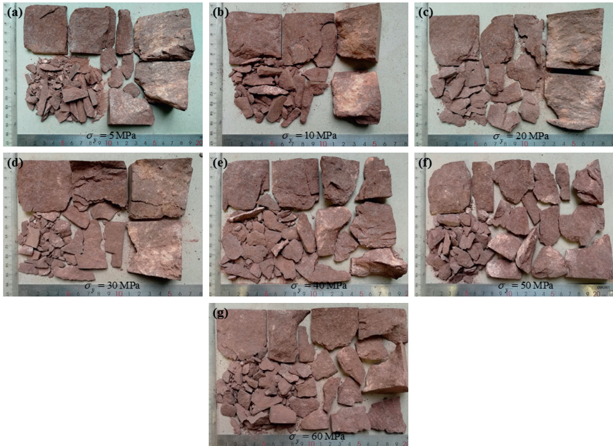
FIGURE 9: Failure characteristics of BCT at different confining pressures.
