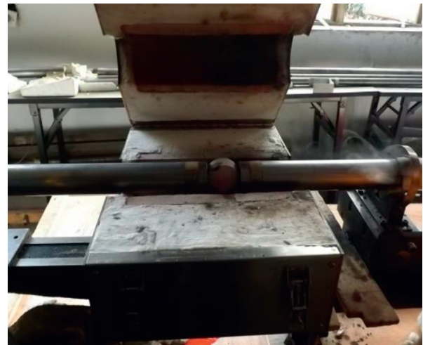
FIGURE 5: Placement of high-temperature sandstone specimen in the dynamic splitting tensile test.
