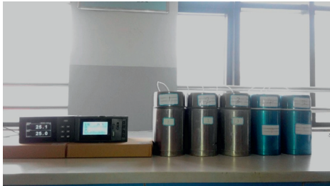
FIGURE 1: Device used to test reaction temperature.
