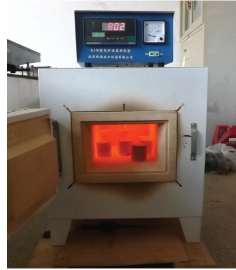
FIGURE 1: Sandstone specimens heated using box-type resistance furnace.
