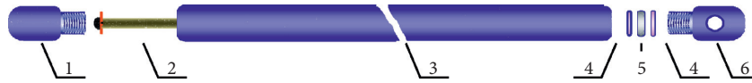
FIGURE 3: Structure of CO 2 cracker. 1, filling valve; 2, heating pipe; 3, main pipe; 4, sealing gasket; 5, shearing piece; 6, energy release head.
