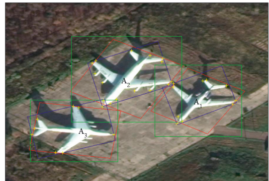
FIGURE 14: RANGE-MBR allows to build quasi-minimum bounding rectangles.
