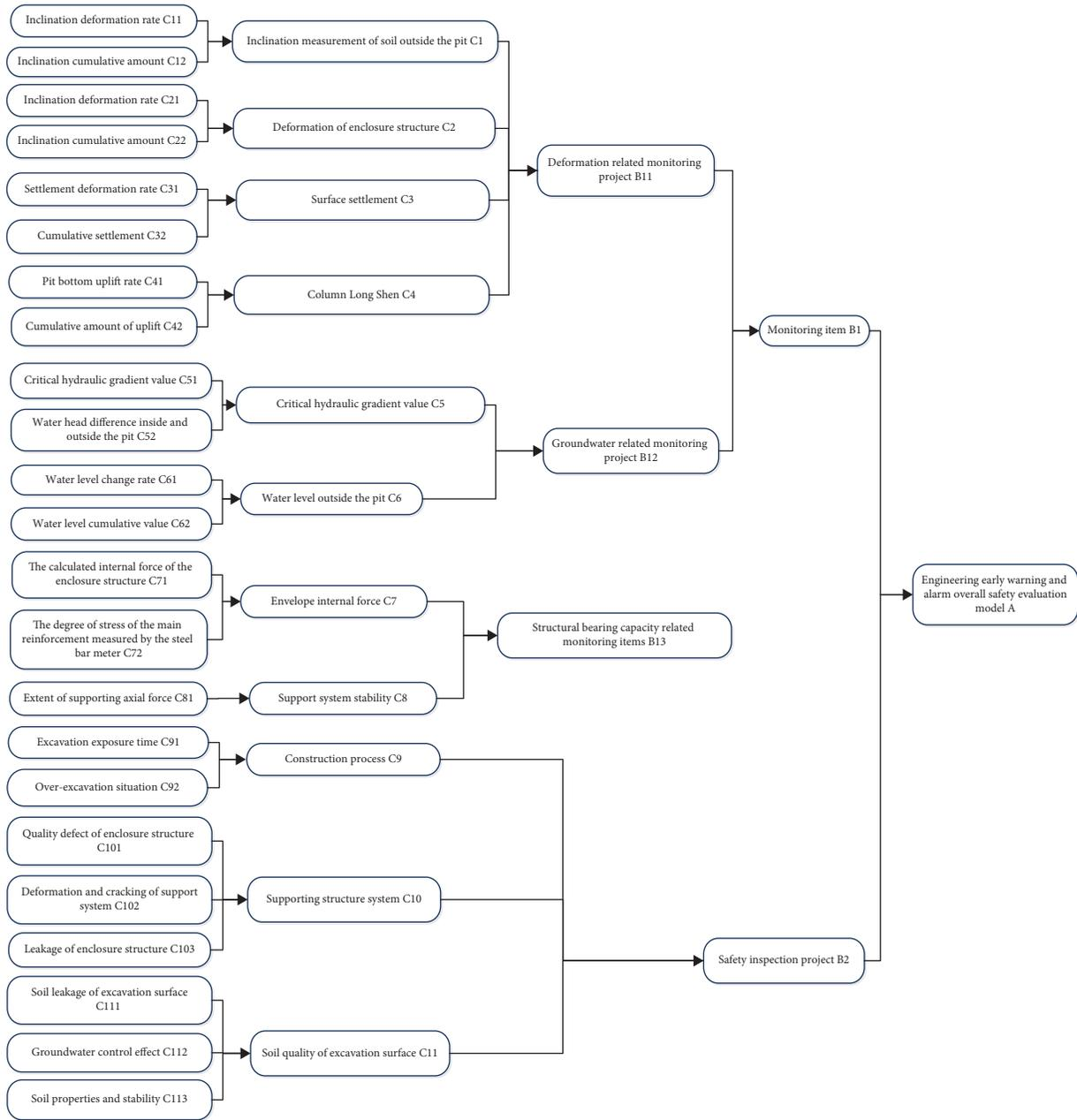
FIGURE 3: Overall safety evaluation model of engineering early warning based on index analysis.
