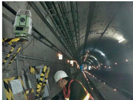
FIGURE 11: Automatic total station and reflection prism.
