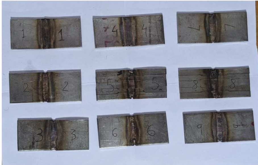
FIGURE 3: Welded joint after the TIG welding.
