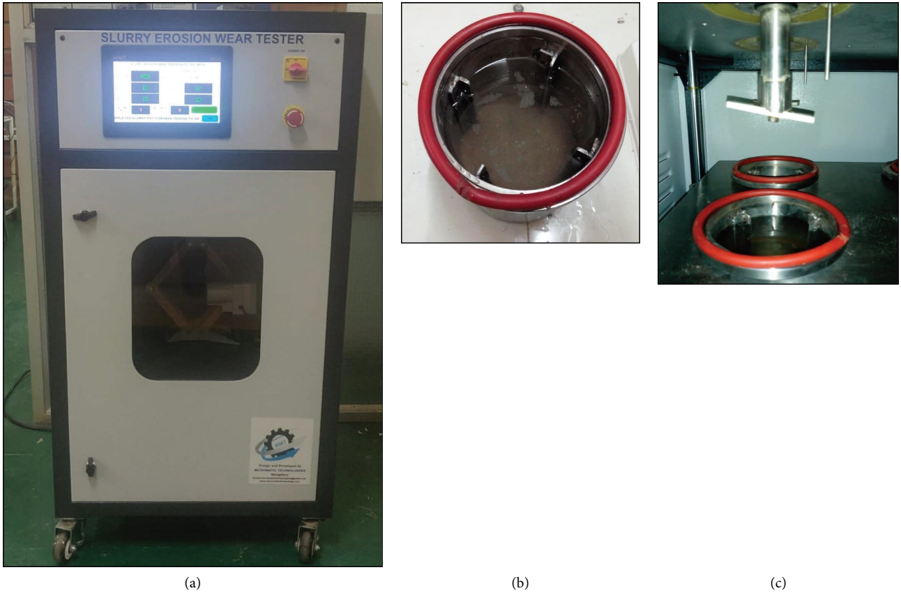
FIGURE 3: Slurry erosion wear test: (a) slurry erosion wear tester, (b) slurry solution, and (c) mounted test specimen.
