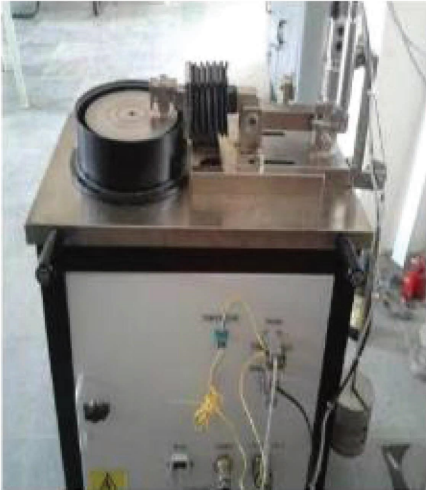
FIGURE 3: Photograph of pin-on-disc machine used for friction and wear test.
