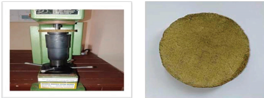
FIGURE 3: Hardness test setup.
