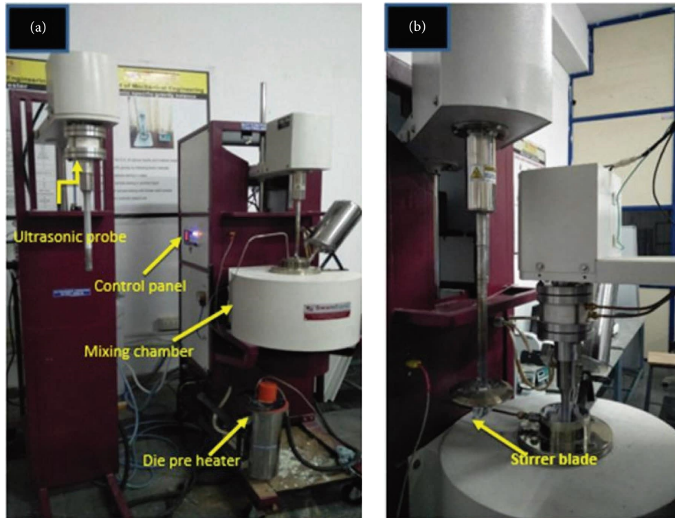
FIGURE 3: Ultrasonic stir casting machine.
