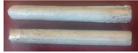
FIGURE 2: Al7049 with B_4C nanometal composite after casting.
