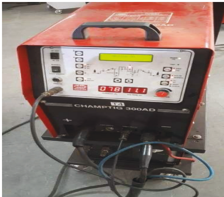
FIGURE 2: TIG welding setup.
