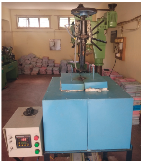
FIGURE 3: Stir casting setup (courtesy: PES College Of Engineering, Mandya).
