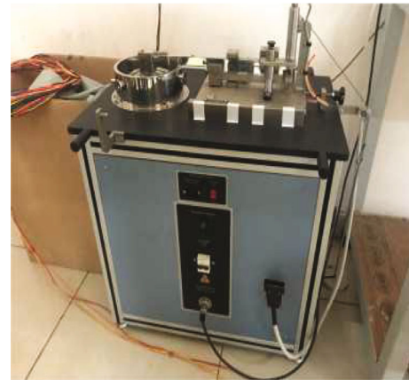
FIGURE 3: Pin on disc apparatus.
