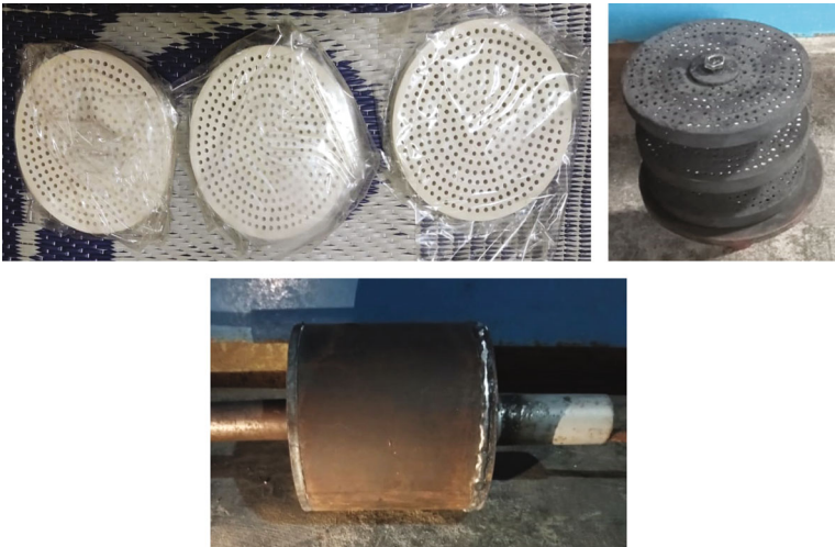
FIGURE 2: Fabrication of SCR catalytic converter.
