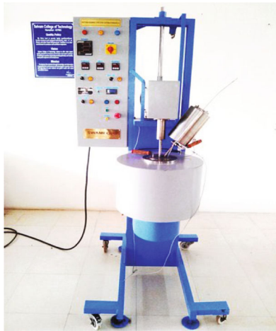
FIGURE 1: Experimental setup of stir casting furnace.
