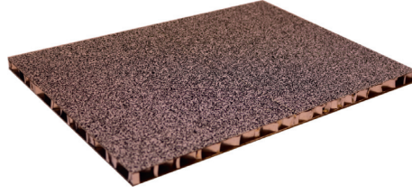
FIGURE 4: Experimental panel with speckle pattern.
