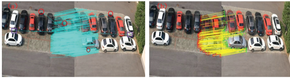
FIGURE 5: Image feature point matching of outdoor parking lot. (a) Traditional SURF algorithm matching. (b) Algorithm matching in this paper.
