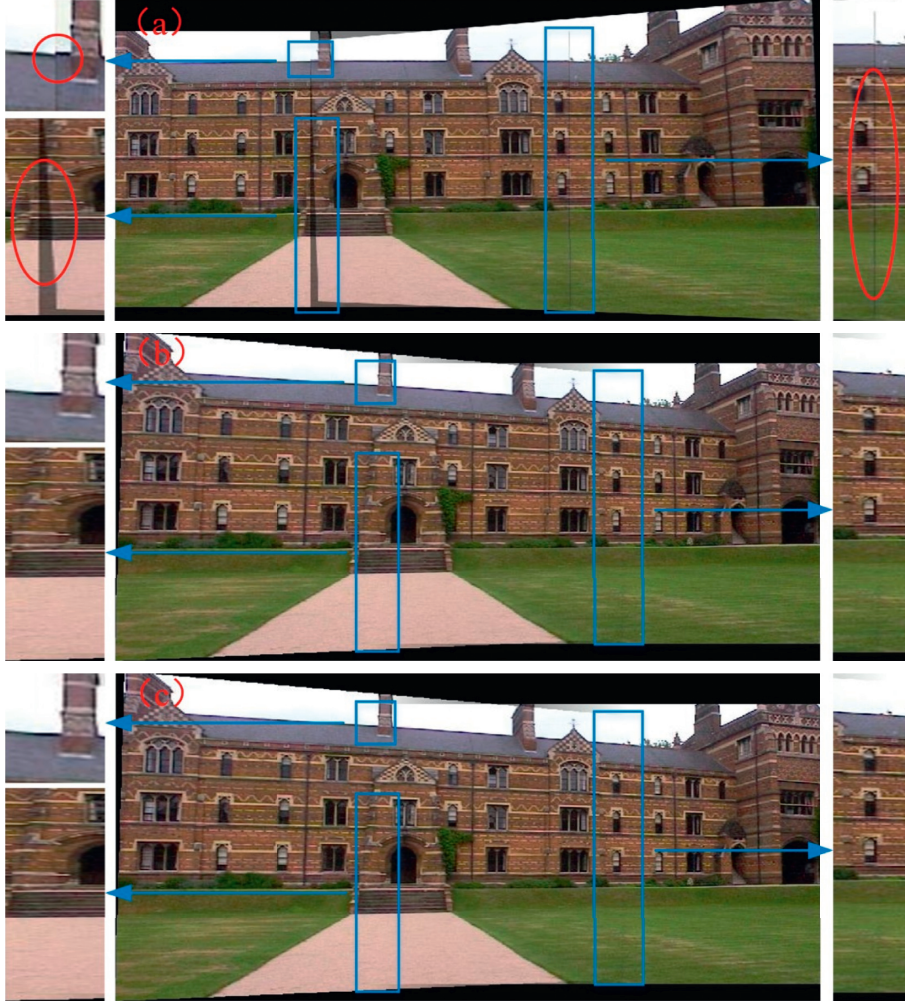
FIGURE 12: Comparison of the results of three fusion algorithms on images with different resolutions. (a) Progressive and progressive weighted fusion algorithm. (b) Fusion algorithm in [23]. (c) The proposed method.
