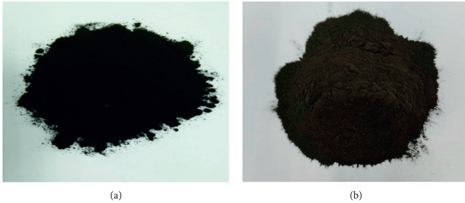
FIGURE 1: Physical appearance of industrial waste powders. (a) Crumb rubber powder. (b) Tin slag.
