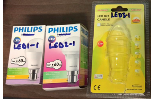
FIGURE 6: Experiment LED lamps. We show three of the lamps with the fourth being LED1-2 having the same power specification as LED1-1 and LED2-1.
