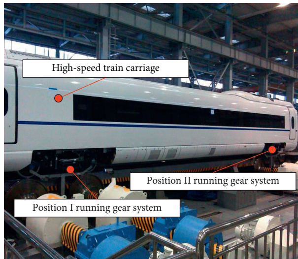
FIGURE 6: Actual position of the running gear system.
