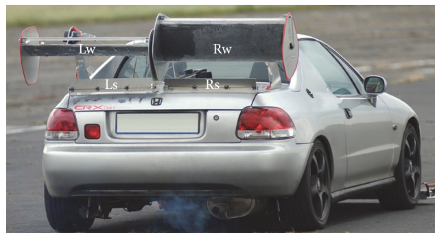
FIGURE 22: Snapshot from a test drive with the active aerodynamics deployed, where Lw/Rw – active left/right wing, Ls/Rs – active left/right spoiler.
