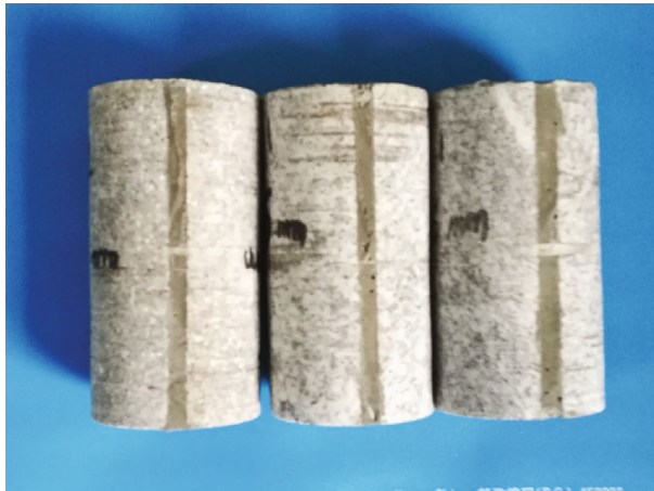
(a) Vertical fissures
