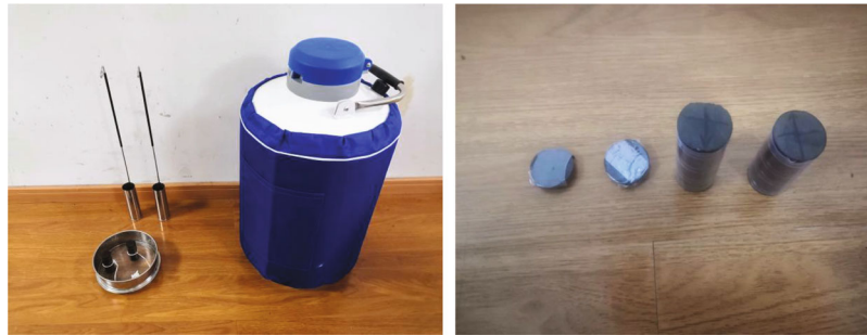
FIGURE 5: Liquid nitrogen freeze-thaw device and frozen samples.
