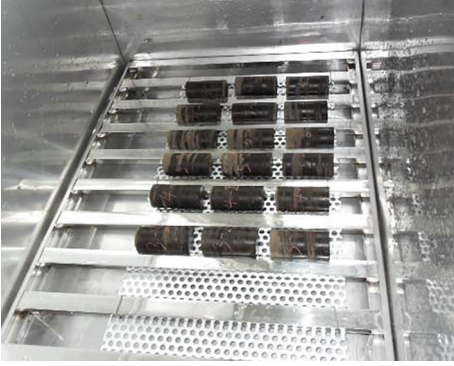
FIGURE 5: Samples in the periodic freeze-thaw experimental apparatus.
