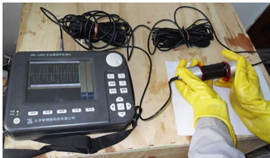
FIGURE 8: Ultrasonic detection on oil shale samples after periodic freeze-thaw cycles.
