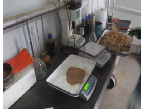
FIGURE 1: Test experiments on the physical properties of quicksand in the water gushing section of the tunnel.
