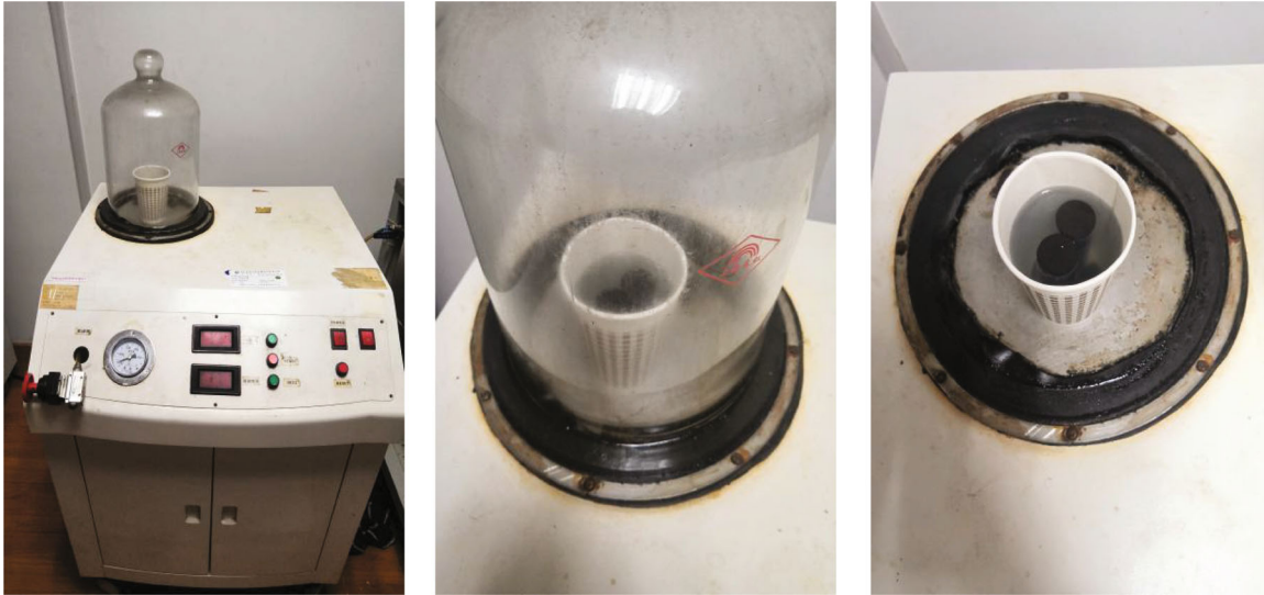
FIGURE 4: Vacuum-water saturation device.
