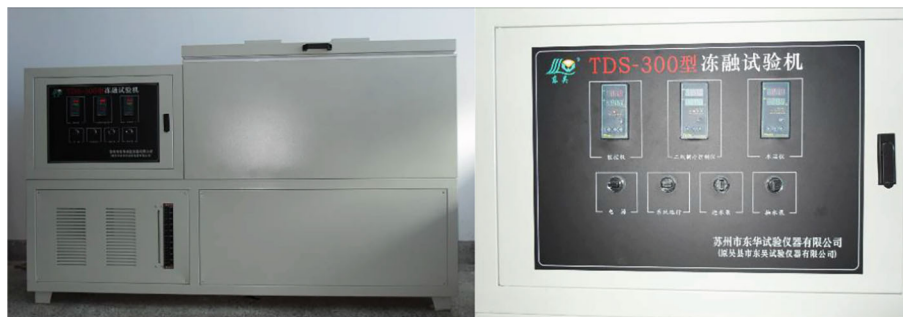
FIGURE 3: Experimental apparatus of TDS-300 periodic freeze-thaw cycles.
