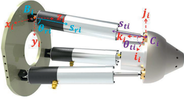
FIGURE 9: Schematic diagram of revolute joint and spherical joint.
