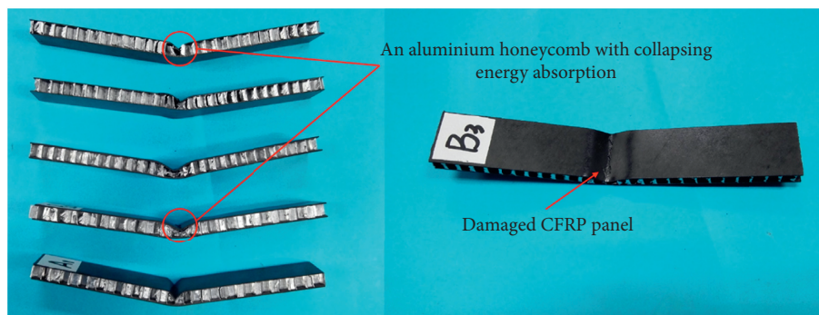
FIGURE 8: Damaged specimens after quasistatic bending.
