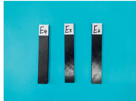
FIGURE 6: Specimens before quasistatic three-point bending test with different loading speeds.
