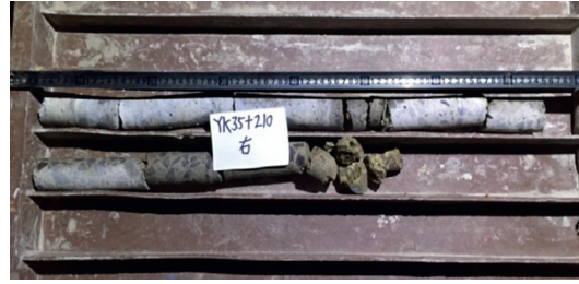
FIGURE 15: Core samples from the surrounding rock and concrete.
