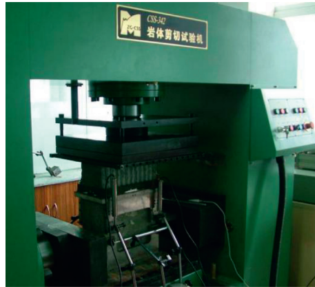
FIGURE 5: The main engine of the rock mass direct shear apparatus.
