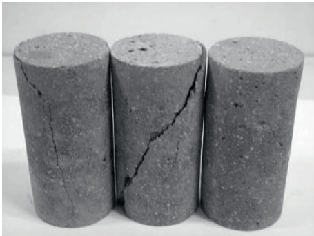
FIGURE 3: Specimens after the compressive strength test.
