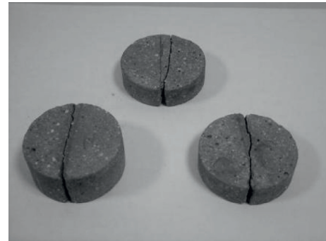
FIGURE 4: Specimens after the tensile strength test.
