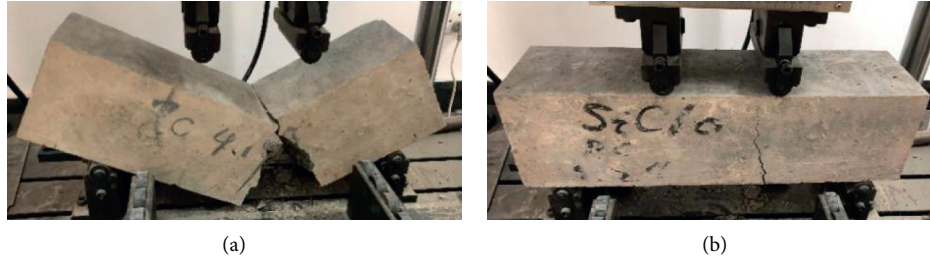
FIGURE 3: Failure morphology of specimens.
