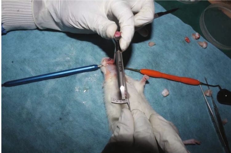
FIGURE 5: Photograph showing torque wrench (range 0-70 N) and an implant hex drive with head specially customised according to the head of the implant screw.
