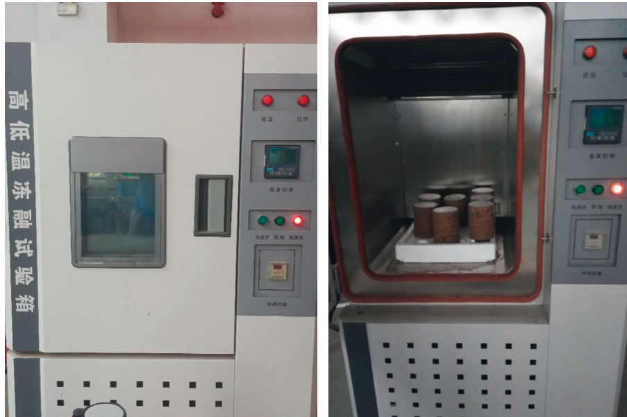
FIGURE 12: Freeze-thaw cycle test.
