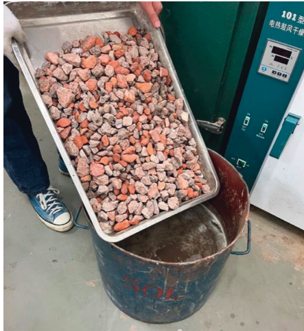
FIGURE 5: PVA solution soaking recycled aggregate.
