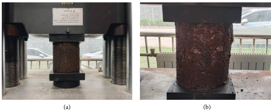
FIGURE 11: Unconfined compression test: (a)Unconfined compression test starts and (b)specimen is crushed.
