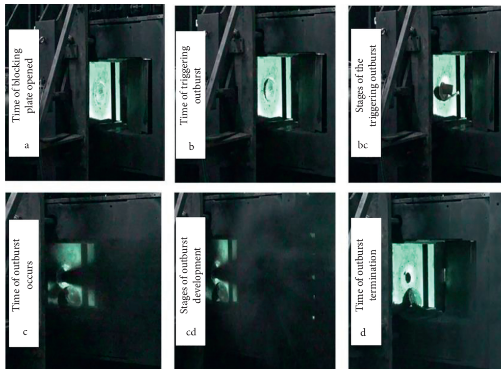
FIGURE 9: Video screenshots of the delay outburst caused by gas accumulation in front of the working face.
