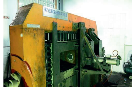
FIGURE 1: Picture of coal and gas outburst simulation system.
