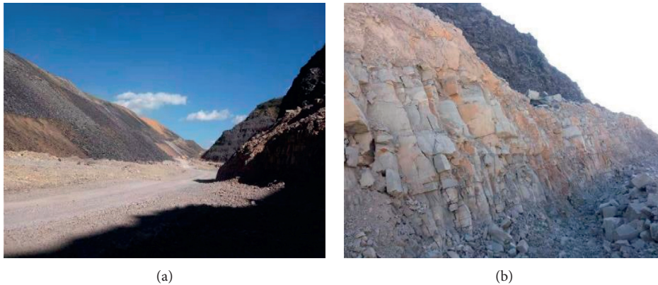
FIGURE 2: The mining status of Jinning Phosphate Mine no. 2 pit. (a) Current status of surface mining. (b) Development of fissures in open-pit mining at this stage.
