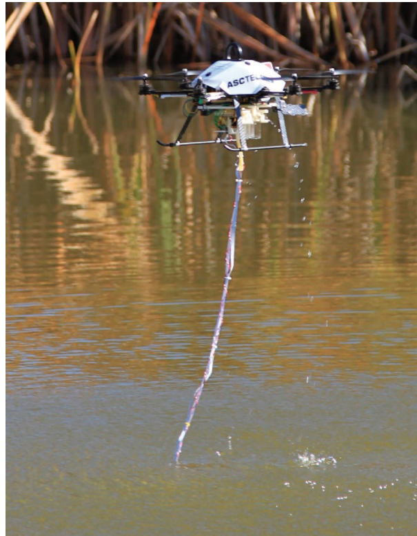
FIGURE 5: Image of UAS-based temperature sampler [96].
