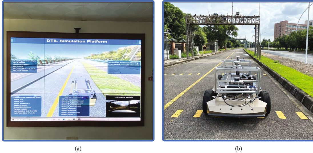
FIGURE 5: Field implementation: (a) DT-assisted simulation platform of car-following test and (b) the AV to be tested drives at the test field.
