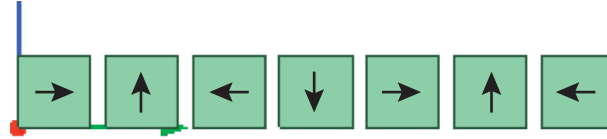
FIGURE 4: Halbach magnet arrangement rule diagram.
