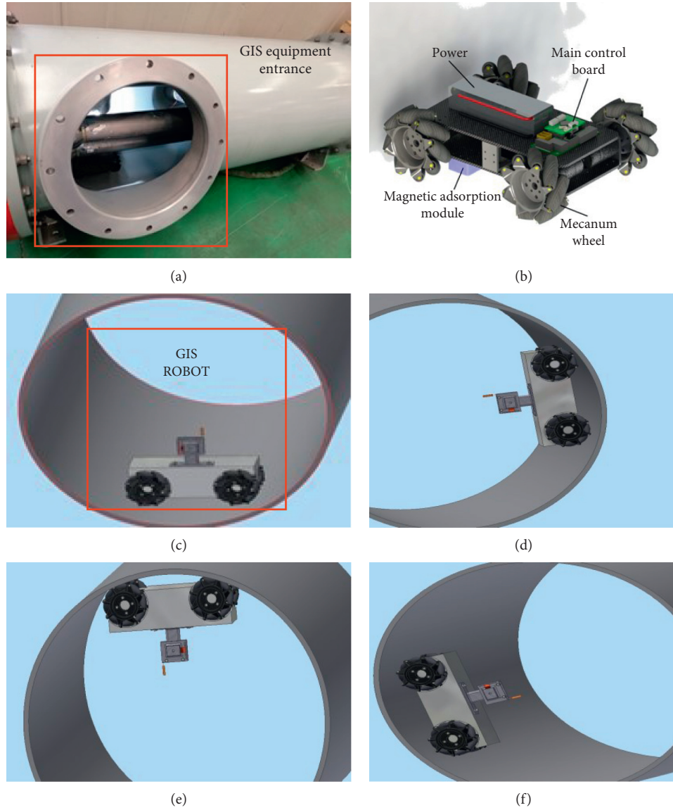
FIGURE 1: GIS equipment inspection robot with adsorption climbing function. (a) GIS operation environment, (b) robot three-dimensional structure, (c) robot inspection status-1 (initial state), (d) robot inspection status-2 (uphill slope), (e) robot inspection status-3 (apical adsorption), and (f) robot inspection status-4 (downhill slope).
