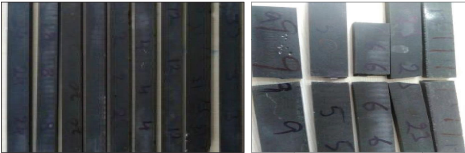
FIGURE 5: Impact test specimens before and after test.
