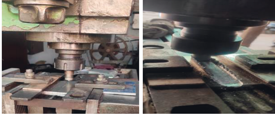
FIGURE 1: Friction stir welding process.
