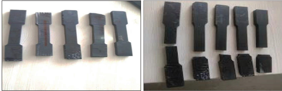
FIGURE 2: Flexural test specimens before and after test.
