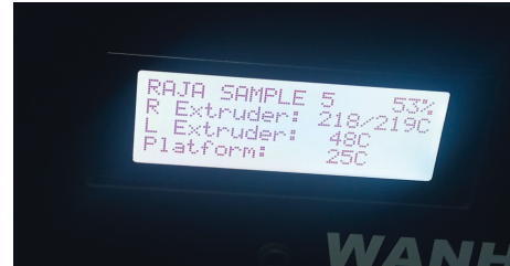
FIGURE 3: Fabrication temperature of the final specimen.
