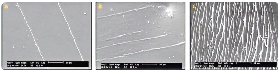
FIGURE 6: Microstructure of neat epoxy, epoxy + 1% Al 2 O 3 and SiO 2 , and epoxy + 3% Al 2 O 3 and SiO 2 .
