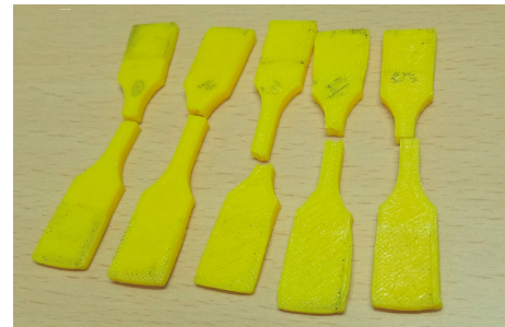
FIGURE 4: Common fabricated samples after the tensile test.
