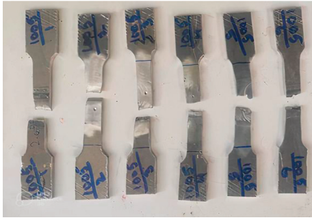
FIGURE 4: Fractured tensile specimens.
