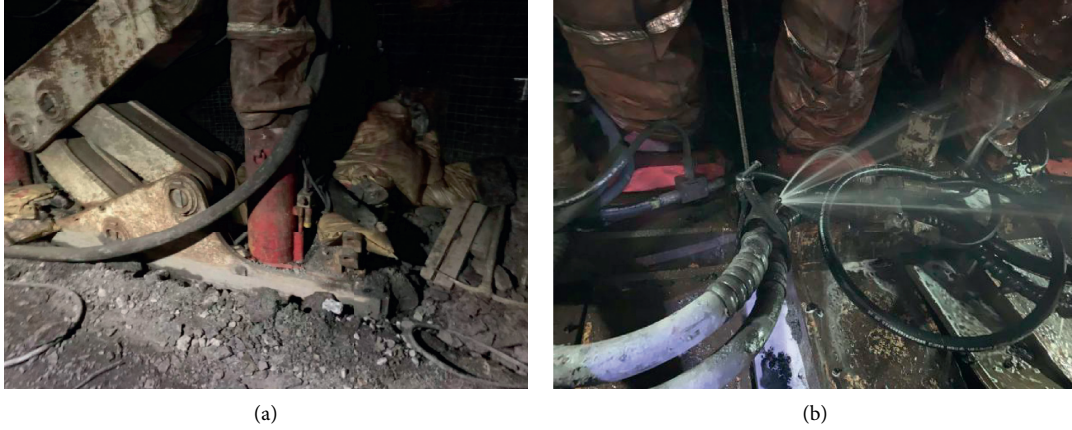
FIGURE 1: A failed support and hydraulic pipe explosion.
