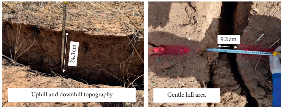
FIGURE 8: Morphological development of surface fissures in shallow seam mining.
