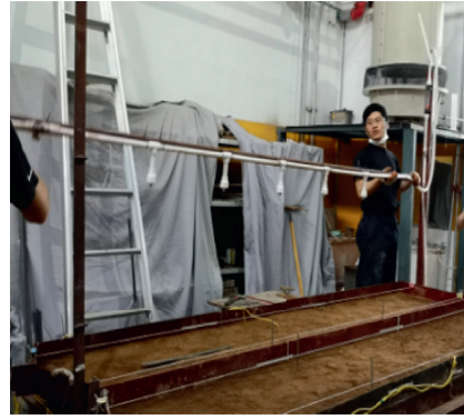
FIGURE 4: Rainfall simulation sprayers installed above the model.
