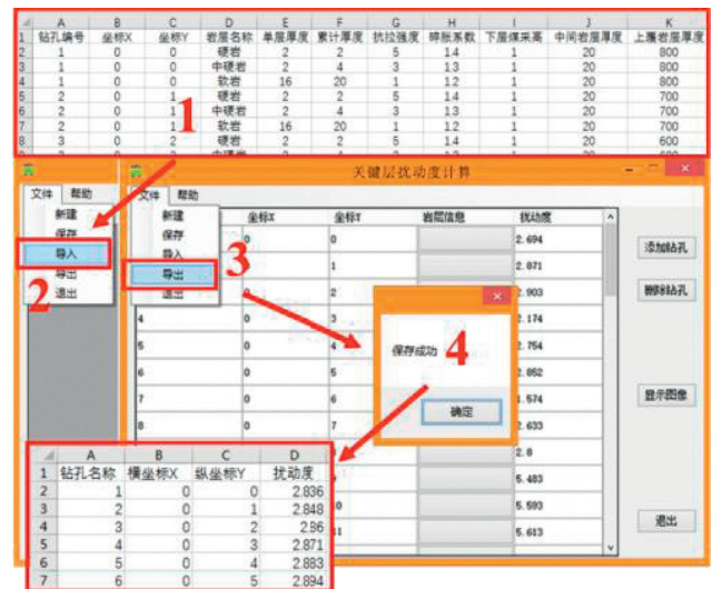
FIGURE 5: Operation flow of batch calculation for KSSD.
