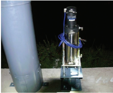
FIGURE 13: Column style installation used in the Beijing-Tianjin and Tianjin-Qinhuangdao high-speed railways.
