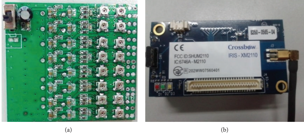
FIGURE 2: (a) Strain sensor board and (b) IRIS mote.
