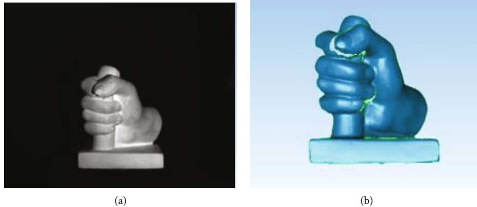
FIGURE 7: Reconstruction results of 3D topography: (a) actual gypsum image and (b) reconstruction result.
