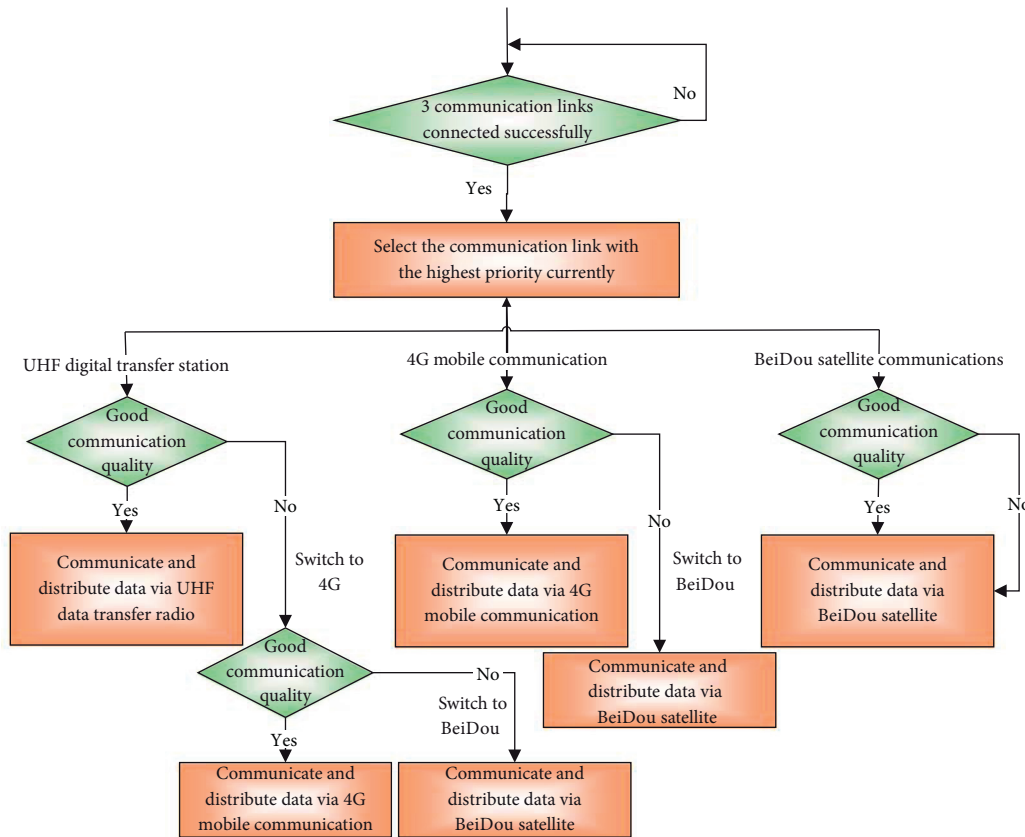
FIGURE 5: Flowchart of multilink adaptation.
