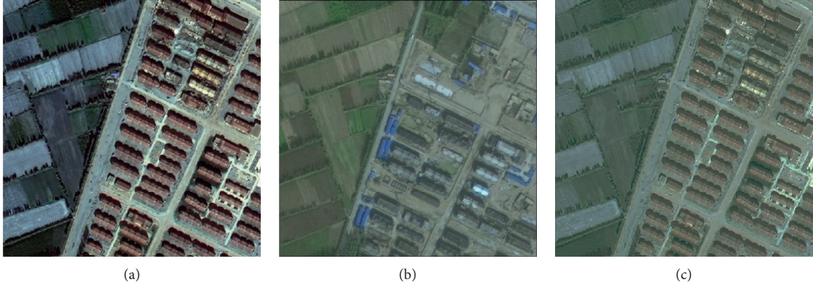
FIGURE 5: Effect before and after histogram matching. (a) The original images of 2017, (b) the original images of 2015, and (c) the processed image of 2017.
