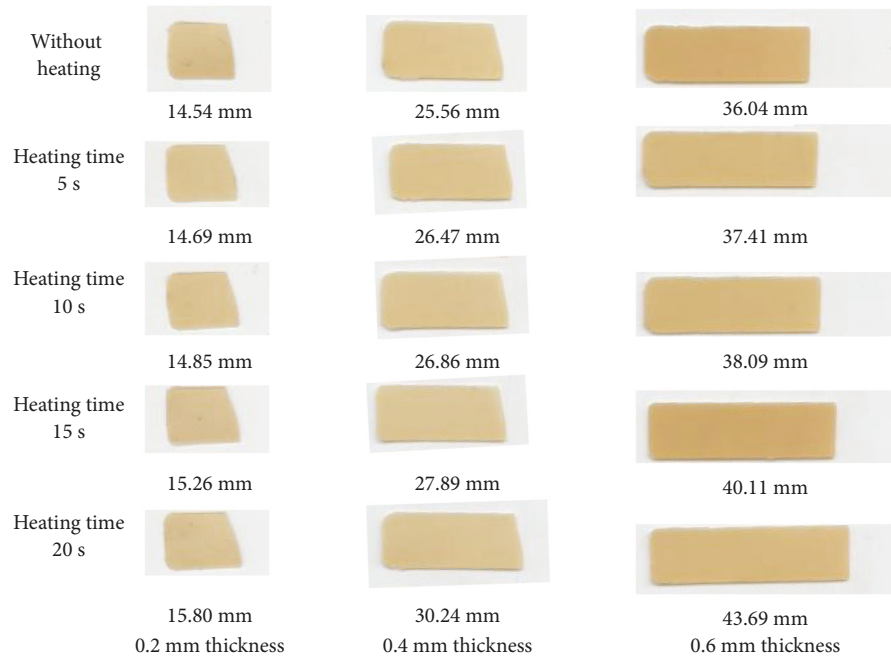
FIGURE 16: Experimental results for melt flow length with the acrylonitrile butadiene styrene material at different heating times.
