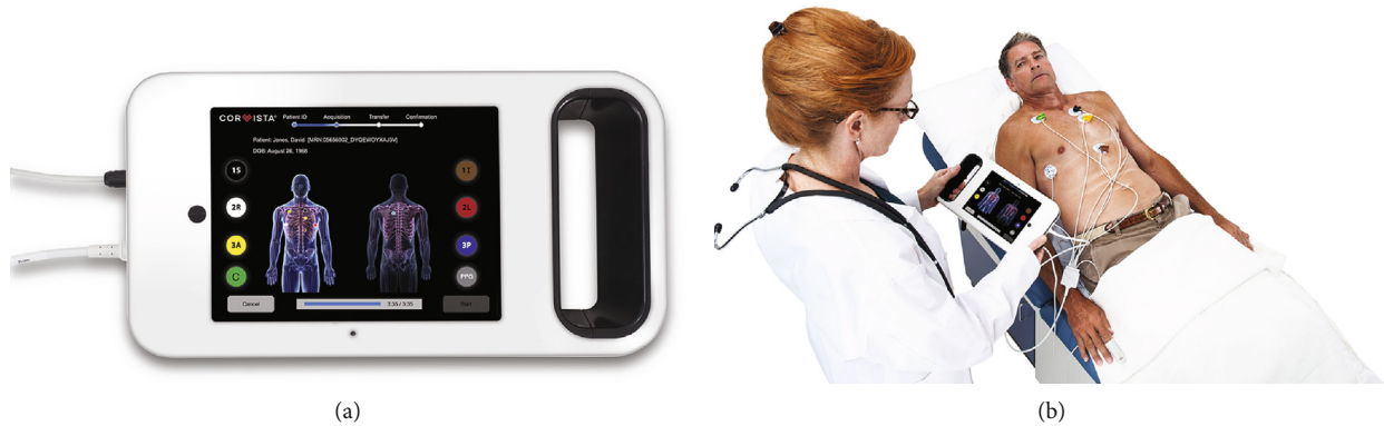
FIGURE 1: Data acquisition setup: (a) signal acquisition device and (b) patient and electrodes/lead placement and PPG configurations.
