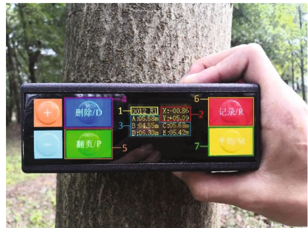
FIGURE 7: Position of the tree. On the display screen, 1 is the tree code and sampling number, 2 is the coordinates, 3 is the distances between the base stations and the mobile station, 4 is the delete key, 5 is the page key, 6 is the record key, and 7 is the average key.
