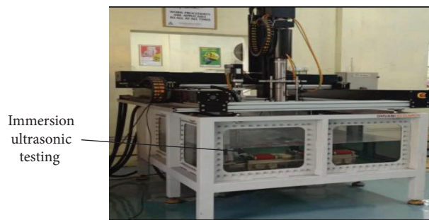
FIGURE 11: Immersion ultrasonic testing system.
