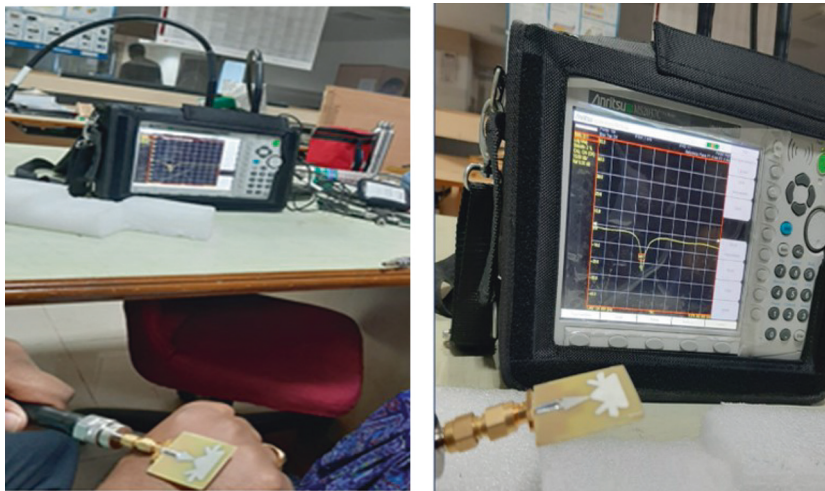
FIGURE 13: Measurement setup using a VNA.
