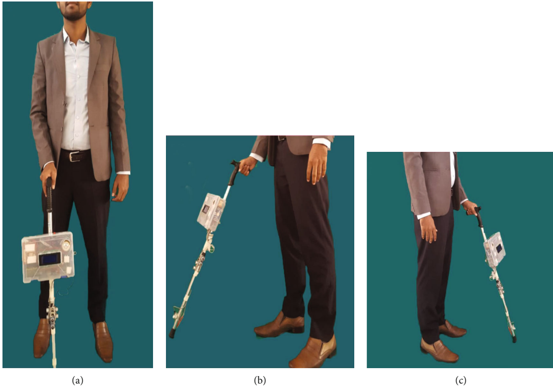
FIGURE 9: Result status diagrams of further enhanced work with an outdoor prototype of the electric guidance cane of visually impaired human. (a) During an outdoor real-time simulation, working on location, GPS and GSM modules were employed to check the longitude and latitude. (b) Display hurdle in front of the first sonar obstacle avoidance sonar sensor: turn right. (c) Motion in front of the second sonar obstacle avoidance sonar sensor: turn left. Water, road depth, and flame are detected in front of the stick, so a vibrator vibrates and the speaker generates a relevant direction command.
