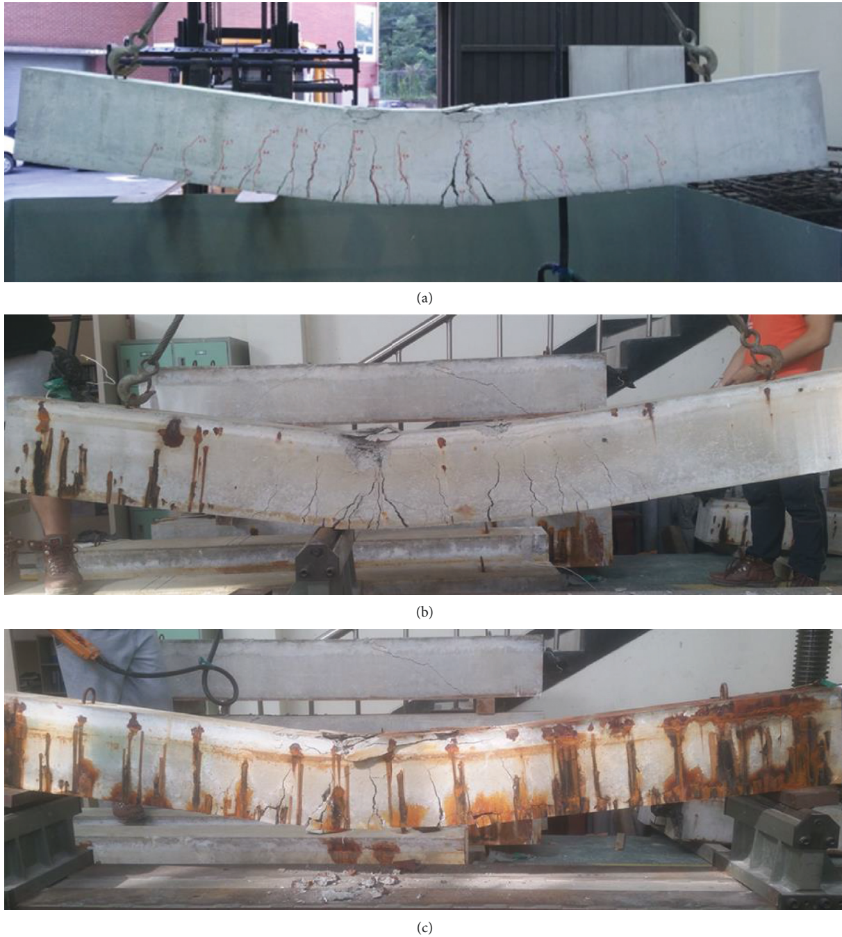
FIGURE 10: Cracking and failure patterns of flexural failure type beams: (a) FB-C0 beam, (b) FB-C4 beam, and (c) FB-C7 beam.
