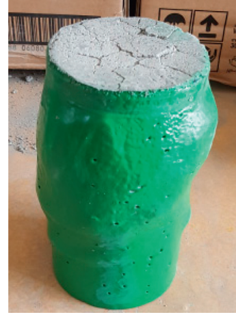
FIGURE 3: Failure mode of polyurea-reinforced concrete cylinder.
