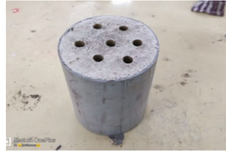
FIGURE 5: PVC pipes as mold cavity.
